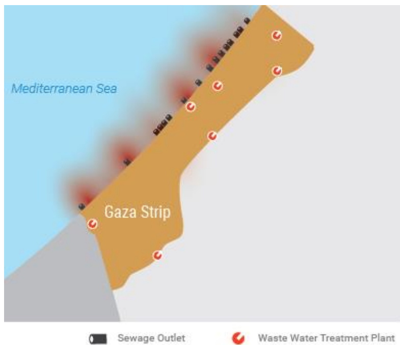
Figure 3.18 Sewage water effluent and sewage treatment plants in Gaza coastline (SP 2020b)
